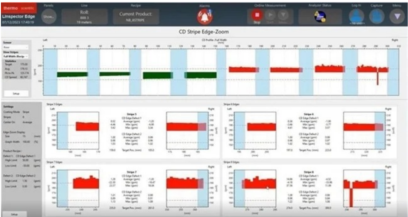
Figure 5. CD stripe edge zoom profiles showing sub-zoom windows for each edge (lower half of the image). Image Credit: Thermo Fisher Scientific – Production Process & Analytics
