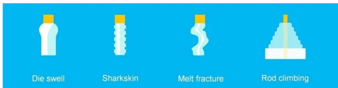
Figure 1. Typical flow anomalies of viscoelastic polymer fluids. Image Credit: Thermo Fisher Scientific – Materials & Structural Analysis
